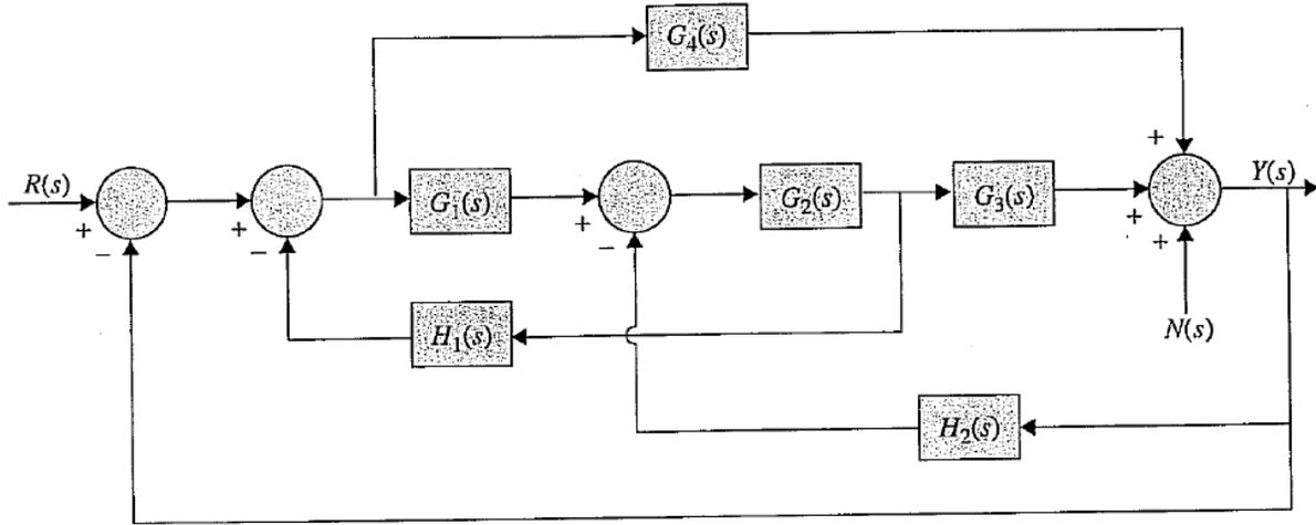
Use the block diagram reduction technique to find the transfer functions
